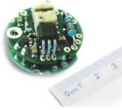
ICA5ATEX ATEX Intrinsically Safe, OEM strain gauge converter, 4-20mA 2 wire
