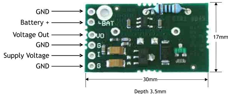
PCB Dimensions: 17 x 30 x 3.5 (height) mm
